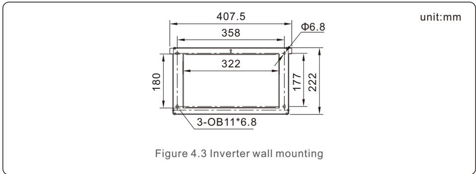
Once a suitable location has been found according to 4.1 using figure 4.3 mount the wall bracket to the wall.
