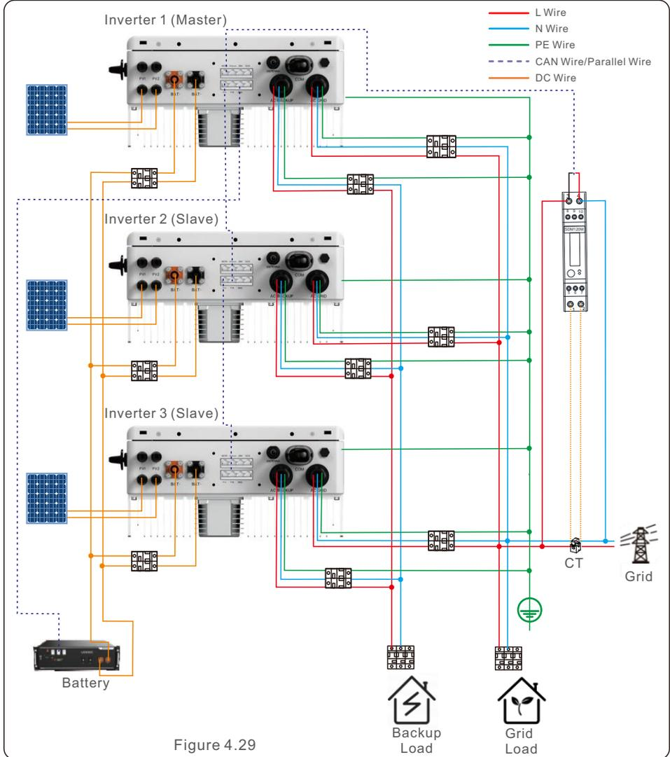
When multiple inverters are connecting in parallel, ONLY same model (same power rating) can be used.
