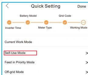
**Self-Use Mode** stores the excess PV power into the battery. If the battery is charged, or there is no battery, the excess PV power will be exported(sold)back to the utility company. If the system is set to not export any power, then the inverter will curtail the PV power(derate the inverter output power).
