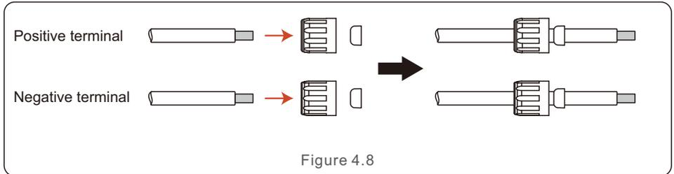
4. Connect the wire part of the DC cable to the metal DC terminal and crimp it with a special DC terminal crimping tool.
