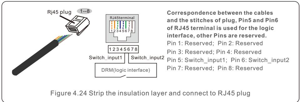
Figure 4.24 Strip the insulation layer and connect to RJ45 plug
