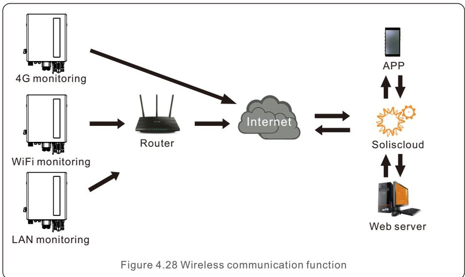
Figure 4.28 Wireless communication function
