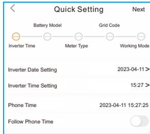
B. Battery Model: Now select the battery model connected to the inverter. This choice must be based on the battery model that is actually connected to the inverter. If there is no battery connected for the moment, select "No Battery" to avoid potential alarms codes.
