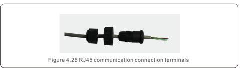
2.Use the network wire stripper to strip the insulation layer of the communication cable. According to the standard line sequence of figure 4.29 connect the wire to the plug of RJ45, and then use a network cable crimping tool to make it tight.
